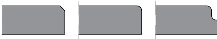
Figure 1.8 – Edge machining. Bevel, rounding and milling.
